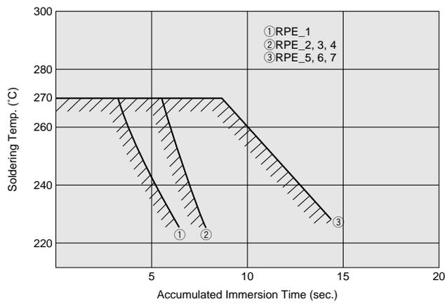
Perform soldering within tolerance range (shaded portion).
