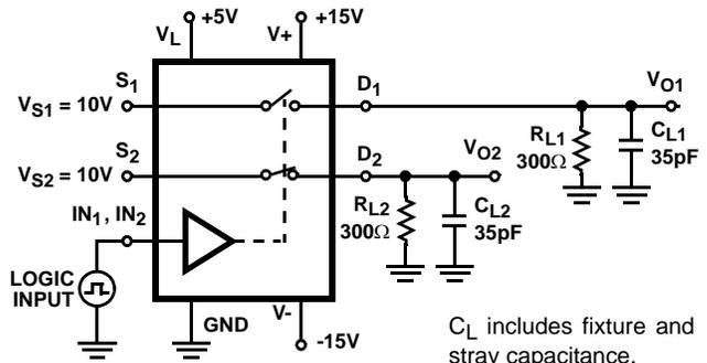
$C_L$  includes fixture and stray capacitance.
