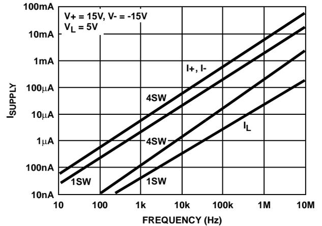
FIGURE 11. SUPPLY CURRENT vs INPUT SWITCHING FREQUENCY
