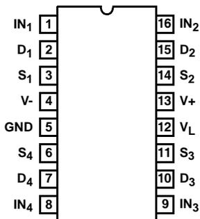
**Functional Diagrams** Four SPST Switches per Package Switches Shown for Logic "1" Input
