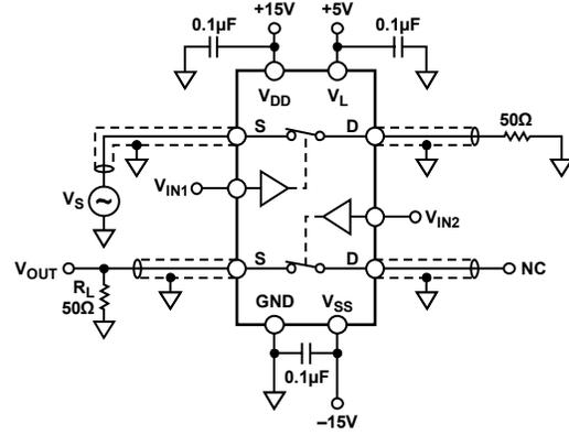
$$\text{CHANNEL-TO-CHANNEL CROSSTALK} = 20 \times \log |V_S/V_{OUT}|$$
