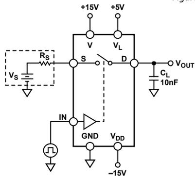
Figure 21. Charge Injection
