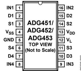
Figure 4. Pin Configuration
