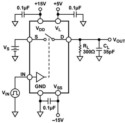
Figure 19. Switching Times
